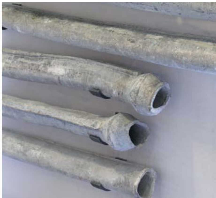
Not a likely source of lead poisoning in New Zealand: Roman lead pipes from the Rhone River. Photo: Ad Meskens http://commons.wikimedia.org/wiki/File:Arles_loden_buizen.jpg
